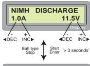
Set discharge current on the left and final voltage on the right. The discharge current ranges from 0.1 to 1.0A and the final voltage ranges from 0.1 to 25.0V). To start the process, press  $\frac{\text{Start}}{\text{Enter}}$  key for more than 3 seconds.
