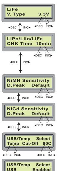
The screen displays the nominal voltage of Lithium battery. There are three kinds of Lithium battery; LiFe(3.3V), Lilo(3.6V) or LiPo(3.7V). This is very important so you have to check the battery carefully and set it up correctly. If it is different from correct value the battery can explode during charge process.
