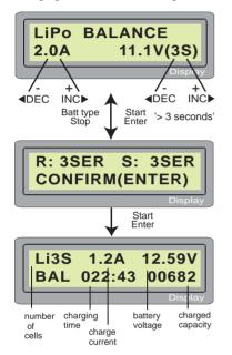
The value on the left side of second line sets a charge current and the value on the right side of second line sets the voltage of the battery pack.
