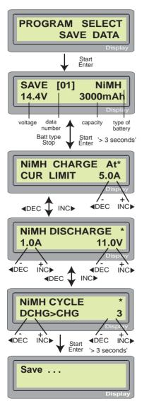
The parameter value setting up in this screen does not affect charge or discharge process. They only represent the specification of the battery. The following screens will automatically be displayed exactly matched with the battery type you set up. The example shows the battery pack of NiMH, 12 cells and 3000mAh of capacity.
