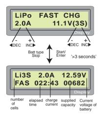
You can set up the charging current and the voltage of the battery pack being charged. As you press Start button the voltage confirmation will be displayed. And then, if you confirm the voltage and current, press Start button again to start charging.
