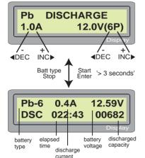
Set discharge current on the left and final voltage on the right. The discharge current ranges from 0.1 to 1.0A. To start the process, press Start key for more than 3 seconds.
